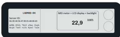
Figure 3: The Eichrecht compliant energy meter display with kWh value and public key
